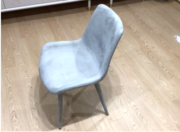
Figure 4. Target object of evaluating 3D reconstruction and viewpoint planing: we used an object which has various shapes, such as the main body's non-convex shapes and thin legs.
